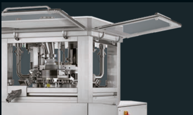
Compact design: In addition to the integrated switch cabinet, space-saving window flaps ensure minimized space requirements with 360° accessibility and largest in class compression chamber.
