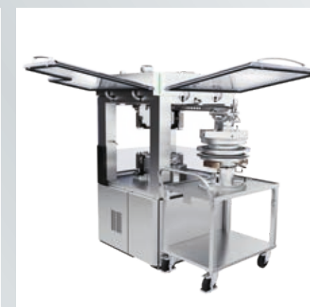
The rotor of the F20i can be changed in just a few minutes using an integrated removal carrier.
