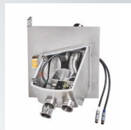
A multi-flexible tablet outlet reduces the risk of material jams.
